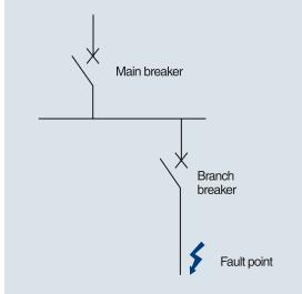
This is an economical approach to the use of circuit breakers, whereby only the main (upstream) breaker has adequate interrupting capacity for the maximum available fault current.
